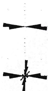
Figure 5. a) Orientation of joints in rocks (Anuradhapura) b) Splitting directions
